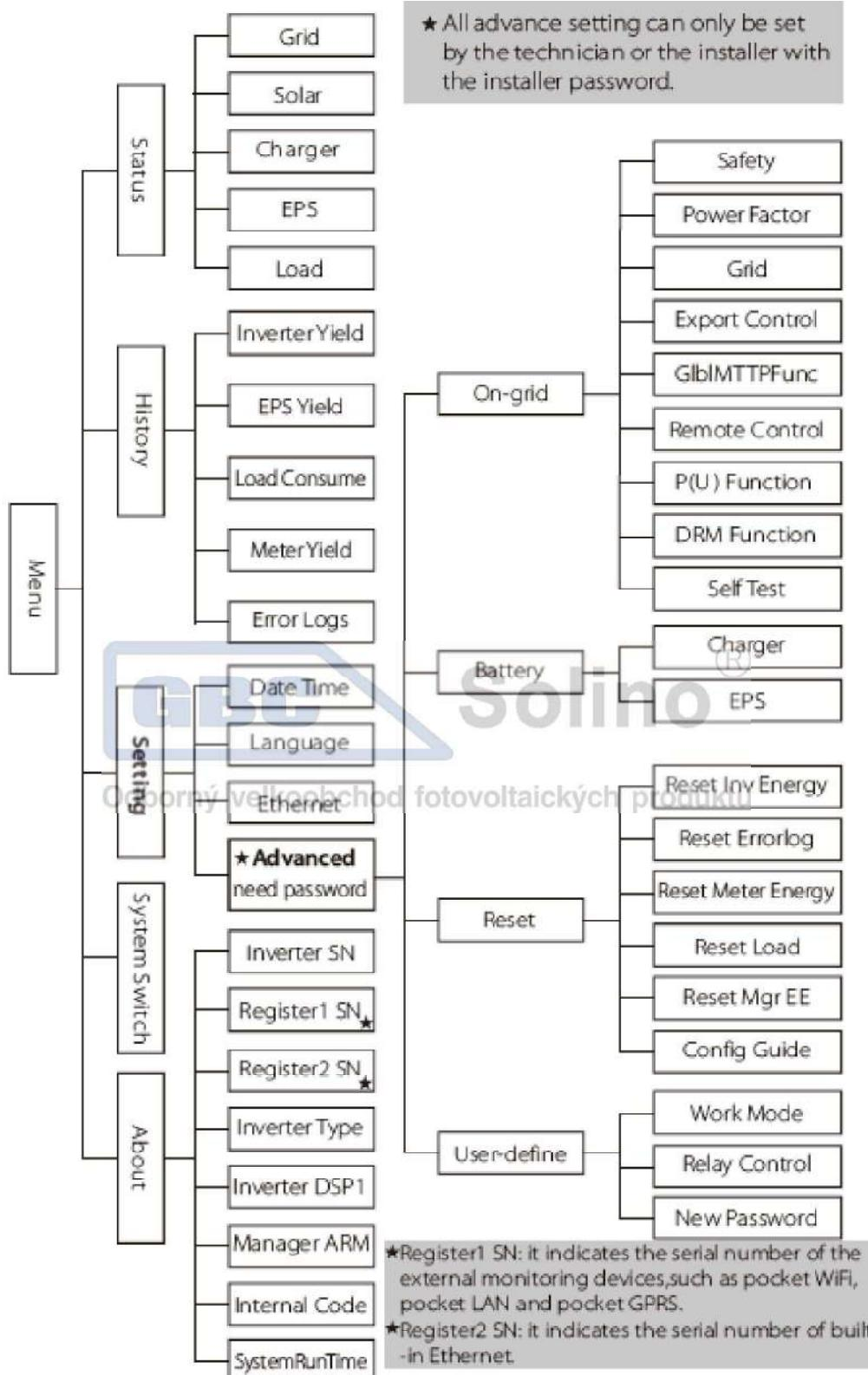
\*Register1 SN: it indicates the serial number of the external monitoring devices,such as pocket WiFi, pocket LAN and pocket GPRS.
